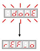
7.Press ENTER key to return to the Fn003 display of the utility function mode.
