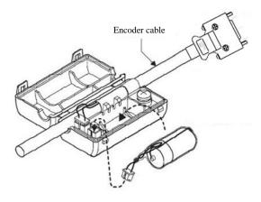
C.Cover the shell of the battery case.
