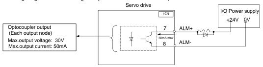
An external +24V I/O power supply is required since there is no +24V power source available inside the servo drive.
