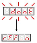
6. Press the ENTER key to return to the utility function mode display Fn003.
