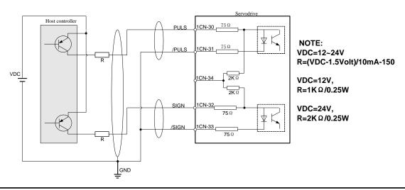
Note: When the host controller is applied by open-collector signal output, the input signal noise margin lowers. When a
