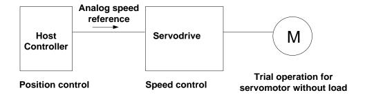
When the servo drive conducts speed control and position control is conducted at the host controller, perform the operation below, following the operation in **Operation Procedure in Speed Control Mode (Pn005=H.**  $\Box\Box\Box\Box\Box$ ).
